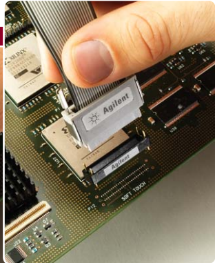
Figure 10. Soft touch connectorless probes have 1/4 the capacitive loading of connector probes and are the industry's most reliable connectorless solution.
